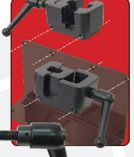
Integra Shocks and Springs is now offering a Universal Compact Shock Vise. This vise can be mounted on either side of the Bench Mount (#310 30205). It is designed for use while working on Piggy Back shocks and features a piston rod clamp.
