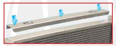
Keyser Manufacturing is now offering a Radiator Hold Down Kit. This kit makes it easy to mount a standard Keyser radiator to the chassis. The top mount of the kit saddles to the top of the radiator and includes: (2) 3/8" threaded tubing drilled and tapped on both ends for 1/4"-20 fittings and (2) straps. Mounting options include using the tubing or welding the straps to the top mount saddle and then bolting to the chassis.
