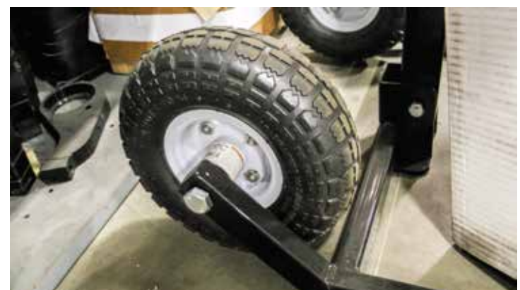
7. Attach wheels to frame.
