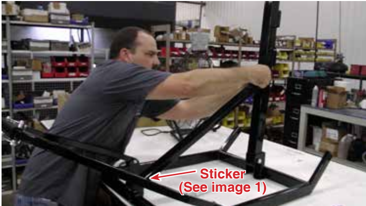
3. Attach brace to front and rear supports, making sure the sticker is facing down and towards the bottom.
