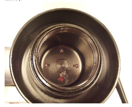
e. Fill the end cap with 80cc of shock oil - p/n: 31030900-1. This should be approximately ½ of the way up to the bottom of the end cap threads. Be sure the alignment balls remain properly seated.
