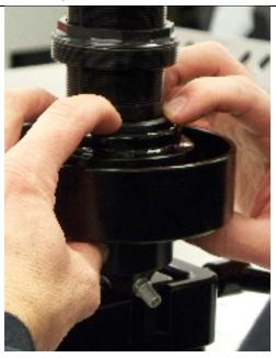
h. Slide the locking ring down until it engages the end cap (as shown below) and tighten the locking ring with the IDA body wrench - p/n: 310 60200. Be sure to hold the pressure tube stationary and allow the locking ring to seat the pressure tube. Tighten only until a slight pressure on the assembly can be felt.
