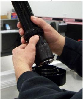
g. Press the bladder base assembly into the cap by applying force through the tube adapter as shown.
