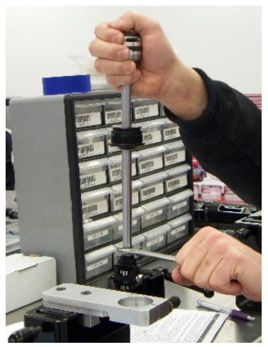
s. Check to see if the adjuster knob rotates freely with the selector shaft in the rebound and then the compression modes. If binding occurs in the compression mode, loosen the jam nut and back the rod end off an additional ¼ turn.
