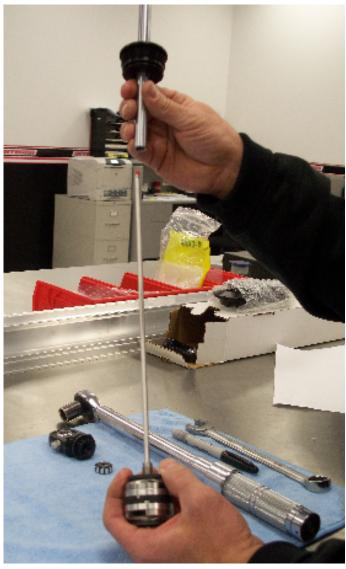
k. Screw the Rod End Assembly - p/n: 310 60030-50 onto the rod end until approximately .100" of the adjuster shaft shows into the window of the rod end. Be sure the selector shaft in the rod end is positioned in the rebound mode "R".
