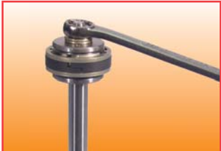
B2 Remove piston nut and washer from the head assembly
