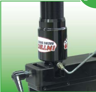
A1 Discharge nitrogen gas prior to disassembly
