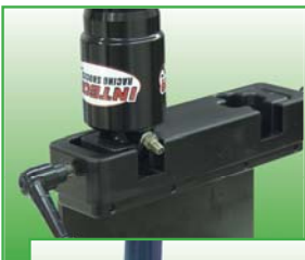
A1 Discharge nitrogen gas prior to disassembly
