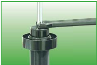
A3 Loosen the rod guide and slowly remove the head assembly
