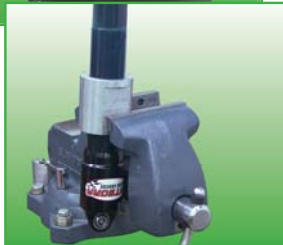
A3 Loosen the rod guide and slowly remove the head assembly
